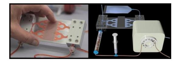
The Wyss Institute's spleen-like blood-cleansing device makes use of genetically modified blood proteins coated on magnetic nanoparticles and magnetic forces to pull a variety of pathogens from the blood. Credit: Harvard's Wyss Institute
