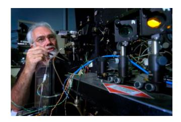
J. Paul Robinson, a Purdue professor of biomedical engineering, makes an adjustment on the multispectral analysis instrument in his laboratory at Discovery Park&acutes Bindley Bioscience Center. With the instrument, Robinson can study 32 colors from a single cell flowing past a laser beam in a fraction of a second, yielding data about cells for applications ranging from medicine to homeland security. Photo: David Umberger
