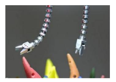
The snake-like robot designed by Johns Hopkins engineers features two thin rods tipped with tentacle-like tools capable of moving with six degrees of freedom. Credit: Will Kirk/JHU
