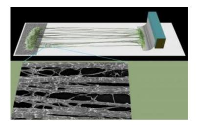
Schematic of stretch-grown axons, showing axons growing on electrodes on right and computer-controlled motor pulling axons to left. Blow-up is close-up of stretch-grown axons. Credit: Douglas H. Smith, MD, University of Pennsylvania School of Medicine
