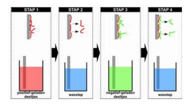
Layer-by-Layer deposition technique. With this technique, ultra-thin DNA layers can be built up and immobilized. The first layer attaches to the surface by means of adsorption. The subsequent layers remain in place due to electrostatic interactions. This makes it possible to build up multiple layers with opposite charges. Step 1 positively charged particles, Step 2 washing stage, Step 3 negatively charged particles (DNA), Step 4 washing stage. Credit: NWO
