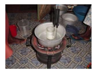
Materials used for the demonstration included cow's milk, a locally purchased glass jar, a locally purchased aluminum pan, and a small charcoal stove that is commonly used for cooking. The temperature probes used in the test are not required in actual practice. Credit: UC Berkeley
