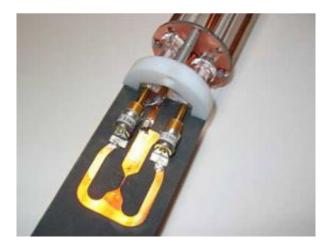
MIT researchers created this NMR probe, which is smaller than a credit card and decreases by several orders of magnitude the amount of a protein needed to measure the protein's structure. Photo courtesy: Yael Maguire
