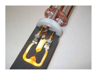
MIT researchers created this NMR probe, which is smaller than a credit card and decreases by several orders of magnitude the amount of a protein needed to measure the protein's structure. Photo courtesy: Yael Maguire
