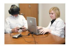
The DETECT system includes an LCD display in a visor with an onboard dedicated computer, noise reduction headphones and an input device (controller).
