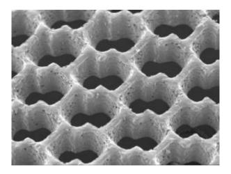
Scanning electron micrograph of an accordion-like honeycomb scaffold for cardiac tissue engineering. Original magnification =100 X Photo courtesy / G.C. Engelmayr, Jr
