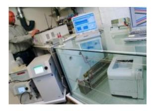
In a test chamber, researchers investigate what kind of particles laser printers release into the ambient air. Image credit: Fraunhofer WKI.
