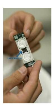
Surgicam - a layer of the current prototype of SurgiCam; blue arrow points to area where the lens module will be seated. [SurgiCam Team Photo Gallery]
