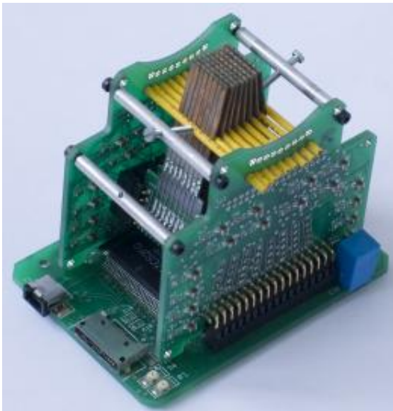
Piezoelectric tactile stimulator. Courtesy Jerome Pasquero, McGill University
