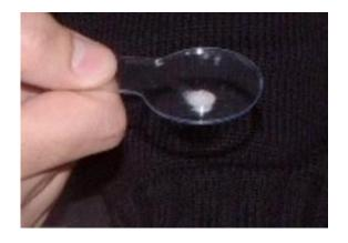
This is the original okay-to-kiss device, containing a color indicator and saliva collector. Credit: AFTAU
