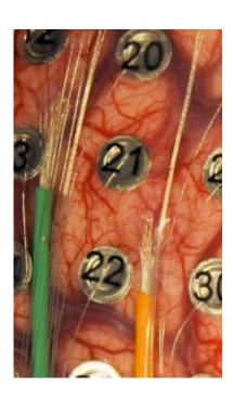
Microwires emerging from the green and orange tubes connect to two arrays of 16 microelectrodes. Each array is embedded in a small mat of clear, rubbery
