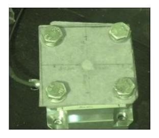
This is a force platform used to study hammering performance. Credit: Duncan Irschick
