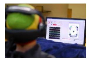
Trial participant Cruise Bogle trains the computer to understand how he will move his tongue to indicate the different commands necessary to operate the powered wheelchair -- forward, backward, right, left and stop. Credit: Georgia
