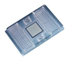
The Fluidigm chip analyzes tumor cells to isolate them from the blood of patients with prostate cancer. The array comprises a matrix of integrated channels and valves (center) housed in an input frame and can run 9,216 parallel reactions.
