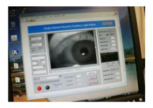
The computerized binocular infrared pulillography device produces a movie and other data that demonstrate how the eye's pupil reacts to a flash of light. Credit: University of Missouri
