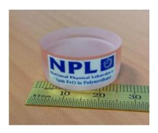
NPL's point spread phantom allows Optical Coherence Tomography instrument manufacturers to align the optical pathways in their machines. This allows them to optimize their performance and ensure that the systems will operate within specification once they are deployed in the field. Credit: Dr Pete Tomlins, NPL
