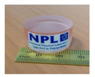
NPL's point spread phantom allows Optical Coherence Tomography instrument manufacturers to align the optical pathways in their machines. This allows them to optimize their performance and ensure that the systems will operate within specification once they are deployed in the field. Credit: Dr Pete Tomlins, NPL
