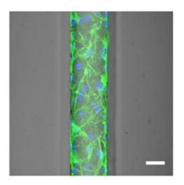
Combined image of a microscopic-phase contrast image of a microfluidic channel (100 micrometres wide) with endothelial cells that have been grown in this channel.
