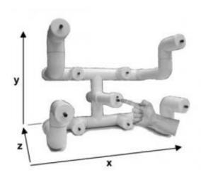
The reaching apparatus used to study the finger paths from a center button to eight other buttons in random order. While volunteers touched the buttons, researchers recorded their brain signals and hand motions. Afterward, the researchers attempted to decode the signals and reconstruct the 3-D hand movements. Credit: Courtesy, with permission: Bradberry *et al. The Journal of Neuroscience* 2010.
