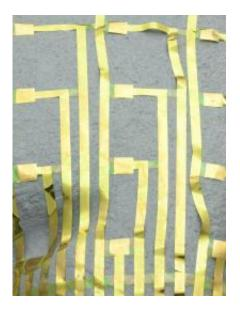
Neural electrode array wrapped onto a model of the brain. The wrapping process occurs spontaneously, driven by dissolution of a thin, supporting base of silk. Credit: Please credit C. Conway and J. Rogers, Beckman Institute
