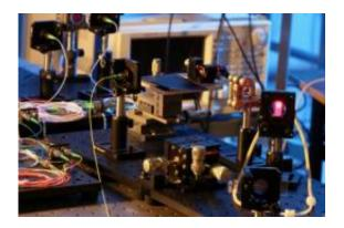
Pictured is an interferometer used in the experimental system developed in Kirill Larin's lab, called Optical Coherence Tomography technique. Credit: Mark Lacy
