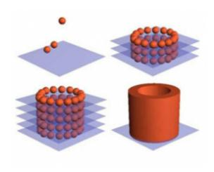
Representation of how bioprinting technology lays down cell aggregates for the fabrication of human tissue. Credit: Organovo via CNET News.
