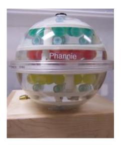
Phannie is the first "phantom" for calibrating magnetic resonance imaging (MRI) machines that is traceable to standardized values. The plastic sphere is about the size of a person's head and filled with 100 smaller spheres used as contrast-enhancing agents and measurement reference markers. NIST researchers in Boulder, Colo., built Phannie, and tested it on an MRI scanner at the University of Colorado Brain Imaging Center. Credit: S. Russek/NIST
