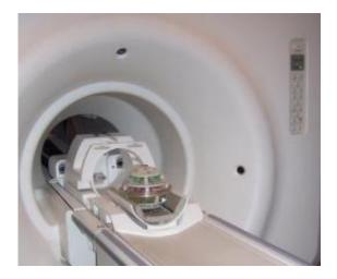
Phannie is the first "phantom" for calibrating magnetic resonance imaging (MRI) machines that is traceable to standardized values. The plastic sphere is about the size of a person's head and filled with 100 smaller spheres used as contrast-enhancing agents and measurement reference markers. NIST researchers in Boulder, Colo., built Phannie, and tested it on an MRI scanner at the University of Colorado Brain Imaging Center. Credit: S. Russek/NIST
