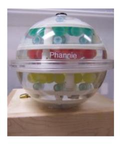
Phannie is the first "phantom" for calibrating magnetic resonance imaging (MRI) machines that is traceable to standardized values. The plastic sphere is about the size of a person's head and filled with 100 smaller spheres used as contrastenhancing agents and measurement reference markers. NIST researchers in Boulder, Colo., built Phannie, and tested it on an MRI scanner at the University of Colorado Brain Imaging Center. Credit: S. Russek/NIST
