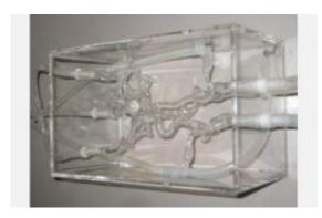
By using silicone copies of human cadaver blood vessels--further modified with aneurisms, atherosclerosis and "plaque"--Insera researchers are able to recreate a model environment for testing their blood-clot removal device. The cadaver model approach could potentially replace some animal testing experiments. Credit: Insera Therapeutics
