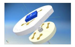
The fiber transmits the laser light to the microscanner mirror. Both are fitted in the tip of the endoscope. (© Fraunhofer IPMS)
