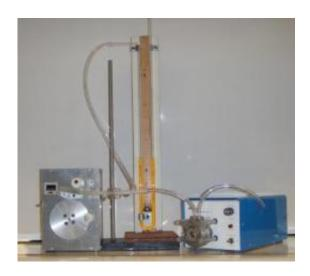
This image shows a smoking machine. From left to right: a puffer box, a manometer, and a pump. Credit: Talbot lab, UC Riverside.
