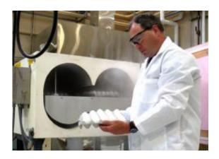
Kevin Keener developed a rapid egg cooling system that uses circulated carbon dioxide to create a thin layer of ice inside an egg's shell that cools the inside of an egg within minutes. (Purdue Agricultural Communication photo/Keith Robinson)
