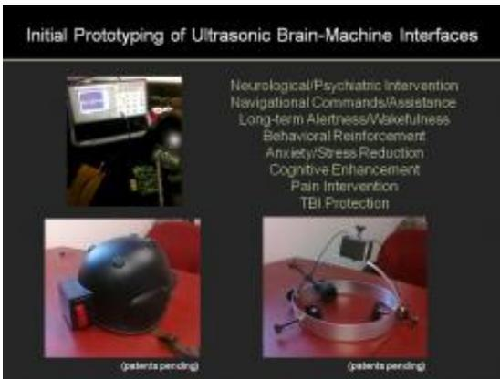
(Lower left) A ballistic helmet fitted with four ultrasound transducers and (lower right) another functional prototype for achieving human brain stimulation using a single element transducer, as well as a list of potential applications relevant to the defense industry. Image credit: Tyler Lab.
