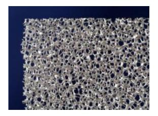
The new titanium-based material features a foam-like structure. Credit: Fraunhofer IFAM
