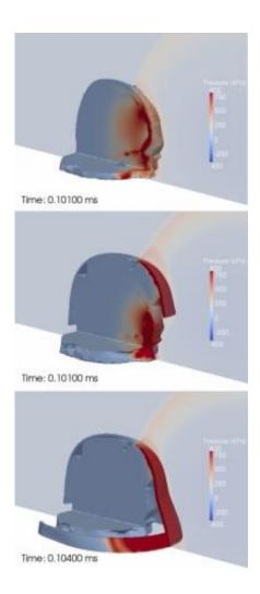
These images show the pressure waves that are transmitted to the brain tissue for the three simulation scenarios considered by Radovitzsky's team: unprotected head (top), head with helmet (middle), and head with helmet and face shield (bottom). The face shield clearly prevents the direct transmission of blast energy into the brain. Images: Michelle Nyein
