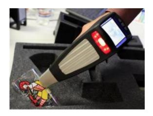
This Sept. 9, 2010 photo shows an Olympus Innov-X Delta Handheld XRF Analyzer testing glassware decorated with a Ronald McDonald character for cadmium, lead and other toxic elements in Los Angeles. The device is used for the analysis of environmental, geological, biological, industrial and other samples. (AP Photo/Richard Vogel)
