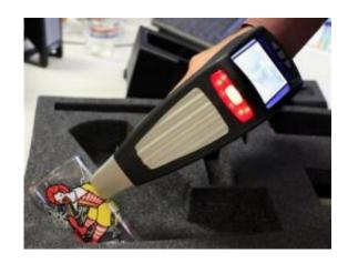
This Sept. 9, 2010 photo shows an Olympus Innov-X Delta Handheld XRF Analyzer testing glassware decorated with a Ronald McDonald character for cadmium, lead and other toxic elements in Los Angeles. The device is used for the analysis of environmental, geological, biological, industrial and other samples. (AP Photo/Richard Vogel)
