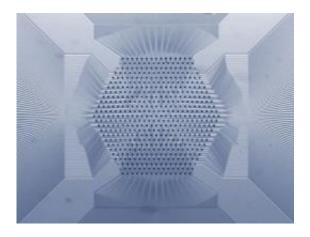
Tiny: The 519-electrode array developed by Dr Mathieson and Dr Gunning at the University of Glasgow's James Watt Nanofabrication Centre.
