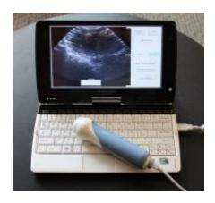
The system uses a hand-held ultrasound probe that connects via a USB port to a touchscreen computer. Credit: University of Washington
