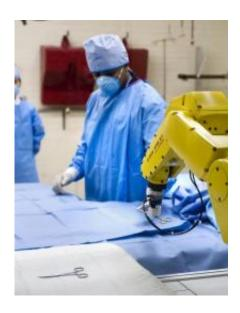
Purdue industrial engineering graduate student Mithun Jacob uses a prototype robotic scrub nurse with graduate student Yu-Ting Li. Researchers are developing a system that recognizes hand gestures to control the robot or tell a computer to display medical images of the patient during an operation. Credit: Purdue University photo/Mark Simons
