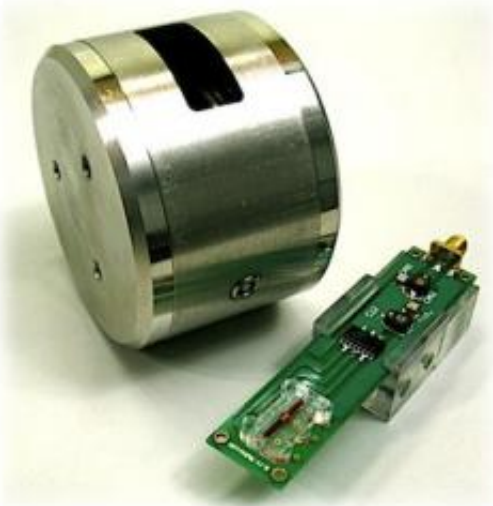
A portable Nuclear Magnetic Resonance device. Image credit: R. Weissleder.
