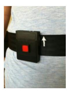
A movement sensor is clipped onto a belt worn around the waist (photo: Stephen Redmond)
