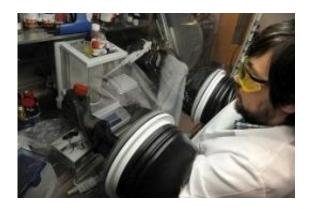
Vanderbilt drug discovery scientist Chris Tarr, Ph.D., prepares for a chemical synthesis in a glove box, which is free of reactive gases such as oxygen and water vapor that can interfere with chemical reactions. Credit: Dana Thomas/Vanderbilt Photography
