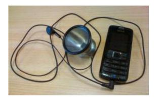
The final prototype: the microphone of a hands-free kit fixed at the base of an egg-cup using blue-tack. A rubber o-ring and a plastic transparency are fixed to the other end to ensure a good seal with the chest.
