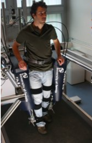
Subject's leg strapped to LOPES exoskeleton
