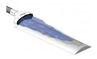
A 3-D rendering of the Air Barrier System area of protection. The blue shaded part represents a 90 percent or greater reduction in airborne contamination over an area approximately 50.8 centimeters (20 inches) long by 15.24 cm (6 inches) wide. The grey zone represents the 80 percent or greater reduction area. Credit: Nimbic Systems, Inc.
