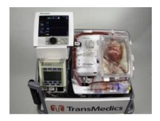
The "heart in a box" device uses a combination of fluid dynamics, software, and preservative solutions to keep a heart beating. Credit: ISNS
