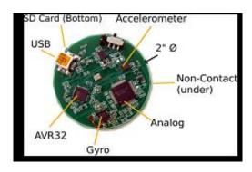
This small device, only about two inches wide, can monitor vital signs while being worn outside the body. (Photo courtesy of Oregon State University)
