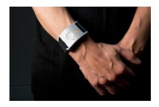
This low-profile wrist sensor, designed by MIT professor Rosalind Picard and her group, has shown early evidence that it can gauge the severity of epileptic seizures as accurately as scalp-worn electroencephalograms EEGs (shown at right). Image: M. Scott Brauer
