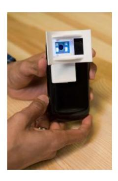
OScan is an ultra-low-cost imaging tool for the oral cavity that attaches to any smartphone's camera, allowing untrained individuals to affordably screen for oral cancer.
