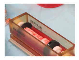
Harvard Bioscience "InBreath" Bioreactor with synthetic laryngotracheal scaffold seeded with patient's own cells
