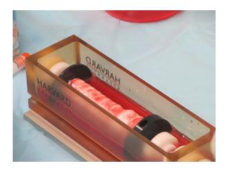
Harvard Bioscience "InBreath" Bioreactor with synthetic laryngotracheal scaffold seeded with patient's own cells
