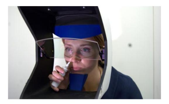
An instrument was used to measure dilation of the pupils and how test subjects focused their gaze while solving tasks on a computer screen in front of them. (Photo: Olga Chelnokova)
