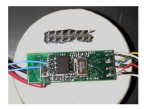
A first-generation transmitter design (white, circular) for measuring and transmitting loads on bone and cartilage in joints is compared to a newer design (green, rectangular) that can be safely implanted into patients. The longer, narrower design is about the length of the diameter of a dime. Credit: UA biomedical engineering department/UA Orthopaedic Research Lab, department of orthopaedic surgery
