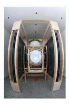
The innovative MEG-MRI device combines the whole-head magnetoencephalography (MEG) and magnetic resonance imaging (MRI) technology. MEG measures the electrical function and MRI visualizes the structure of the brain. Credit: Aalto University
